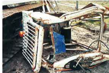
Accident damaged Hitachi KH125-3 crawler crane in our workshop for repair back to new standard.
